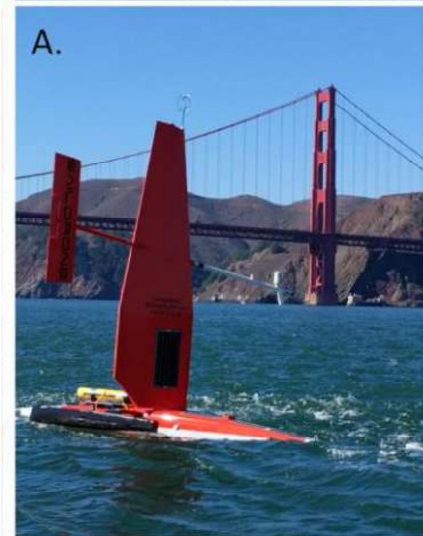
Temporary echosounder installation. A) Saildrone with WBAT (yellow tube) mounted on front. B) Transducer installation on 2 m keel. C) EK60 system mounted in gray box. Alex De Robertis et al, AFSC, NOAA
