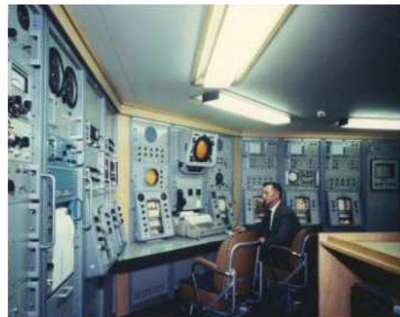
1968 First generation EK scientific echo sounders with calibrated output at 12, 18, 38 and 120 kHz
