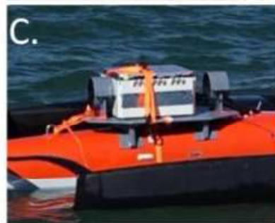
Temporary echosounder installation. A) Saildrone with WBAT (yellow tube) mounted on front. B) Transducer installation on 2 m keel. C) EK60 system mounted in gray box. Alex De Robertis et al, AFSC, NOAA
